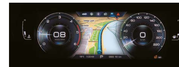
Analogue style instruments with in-cluster navigation
